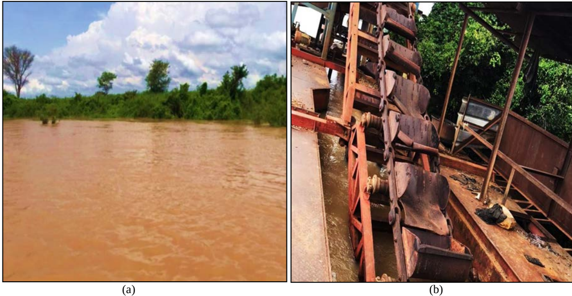
Fig 4: (a) River water laden with fine particles; (b) bucket chain of an abandoned industrial dredge.
